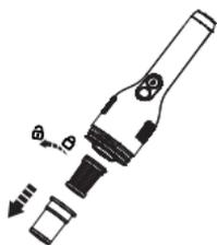
With the dustbin uninstalled, turn counter-clockwise to remove the mesh filter.
